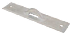
DG01 drill guide with 96mm CC holes and with nibs that fit into 3" CC holes Use for centering 96mm CC holes over 3" CC holes
